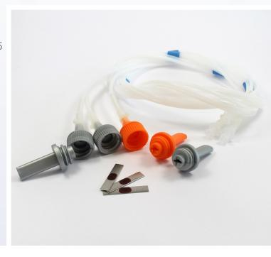
The ParaSure Multi Lumen Channel Control (MLCC) simulates an endoscope with 3 channels (1 x 1mm diameter and 2 x 2mm diameter), providing a unique solution to realistically test the effectiveness of the washer-disinfector. The MLCC combines 3 polypropylene head indicator holders, each of which is connected to a 1.5 metre length of PTFE tubing that terminates in a luer lock.
